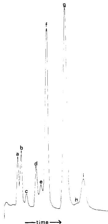
Figure 1. Total ion current vs. time from the MS/GC/COM analysis of the thermolysate (305 min at 175 °C) from 5 plus 8. The products are identified as: a, cis -1,3-diphenylpropene; b, trans -1,3-diphenylpropene; c, cis -1,3-diphenylprop-2-en-1-ol; d, cis -1,3-diphenylprop-2-en-1-one; e, unknown; f, trans -1,3-diphenylprop-2-en-1-ol; g, 3-phenylpropiophenone; h, unknown; and i, trans -1,3-diphenylprop-2-en-1-one.
